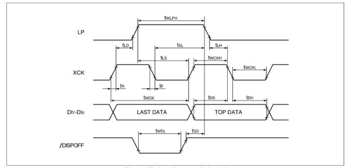
Fig. 6 Timing Characteristics (1)
