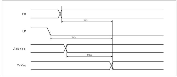
Fig. 8 Timing Characteristics (3)
